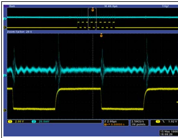
FIGURE 2-40: Digital Feedthrough (SCL signal coupling to V_{OUT} pin); V_{DD} = 5.0\text{V} , V_{REF} = 5.0\text{V} , F_{SCL} = 100\text{ kHz} , V_{OUT} = 20\text{h} ( V_{OUT} Voltage Scale = 20\text{ mV/div} , Time scale = 2\text{ }\mu\text{s / div} ).
