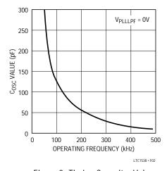
Figure 2. Timing Capacitor Value
