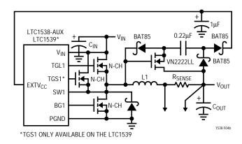
Figure 4b. Capacitive Charge Pump for EXTV<sub>CC</sub>
