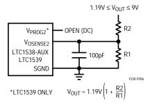
Figure 5b. LTC1538-AUX/LTC1539 Adjustable Applications
