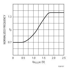
Figure 7. Operating Frequency vs V<sub>PLLLPF</sub>
