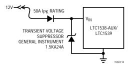
Figure 12. Automotive Application Protection
