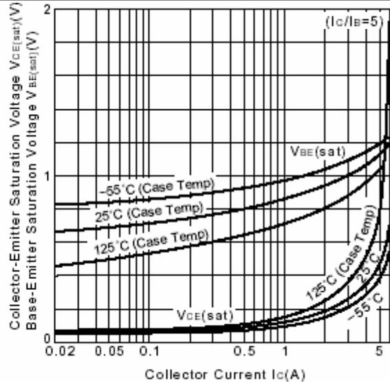
Fig.4 Base-Emitter Saturation Voltage
