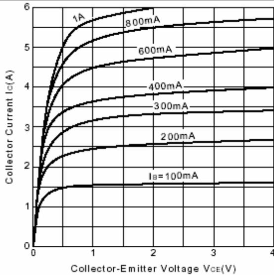
Fig.3 Static Characteristic
