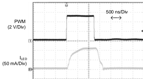
(a) PWM = 150 Hz, Duty = 0.02%, I_{LED} Waveform
