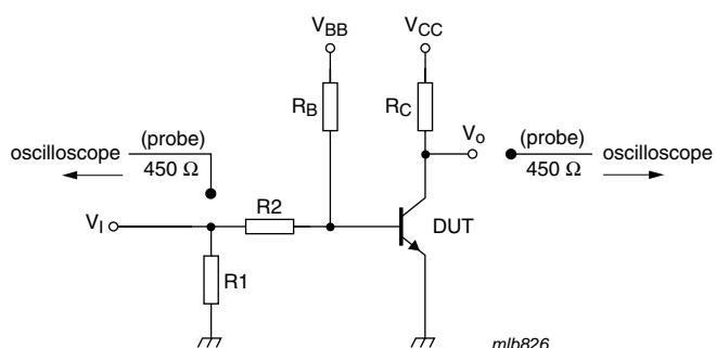
$V_{CC} = 12.5 \text{ V}$ ;  $I_C = 3 \text{ A}$ ;  $I_{Bon} = 0.15 \text{ A}$ ;  $I_{Boff} = -0.15 \text{ A}$
