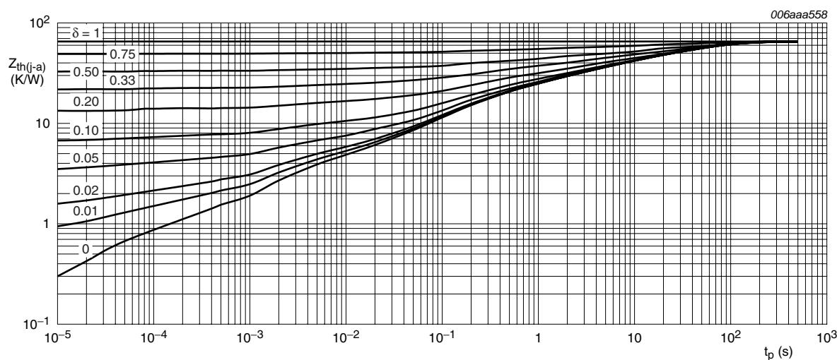
FR4 PCB, mounting pad for collector  $6 \text{ cm}^2$
