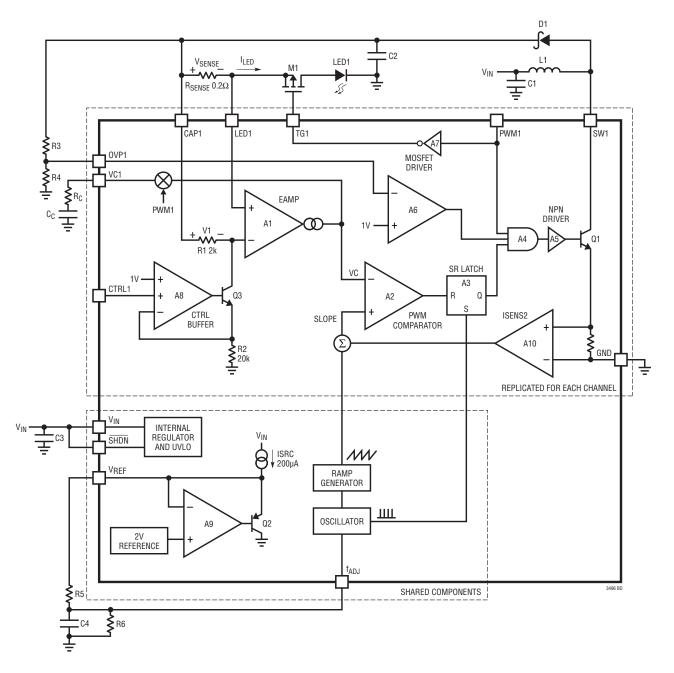
Figure 1. LT3496 Block Diagram Working in Boost Configuration
