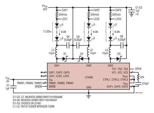
300:1 PWM Dimming at 120Hz
