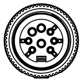
AISG 8-pin female interface with 5 loaded contacts
