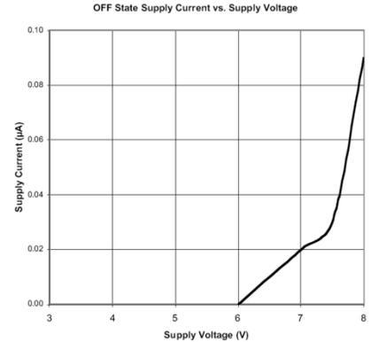
Fig. 9: Off-state Supply Current vs Supply Voltage
