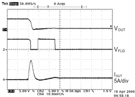
Fig. 20: Short Circuit Transient Response
