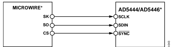
Figure 52. MICROWIRE to AD5444/AD5446 Interface
