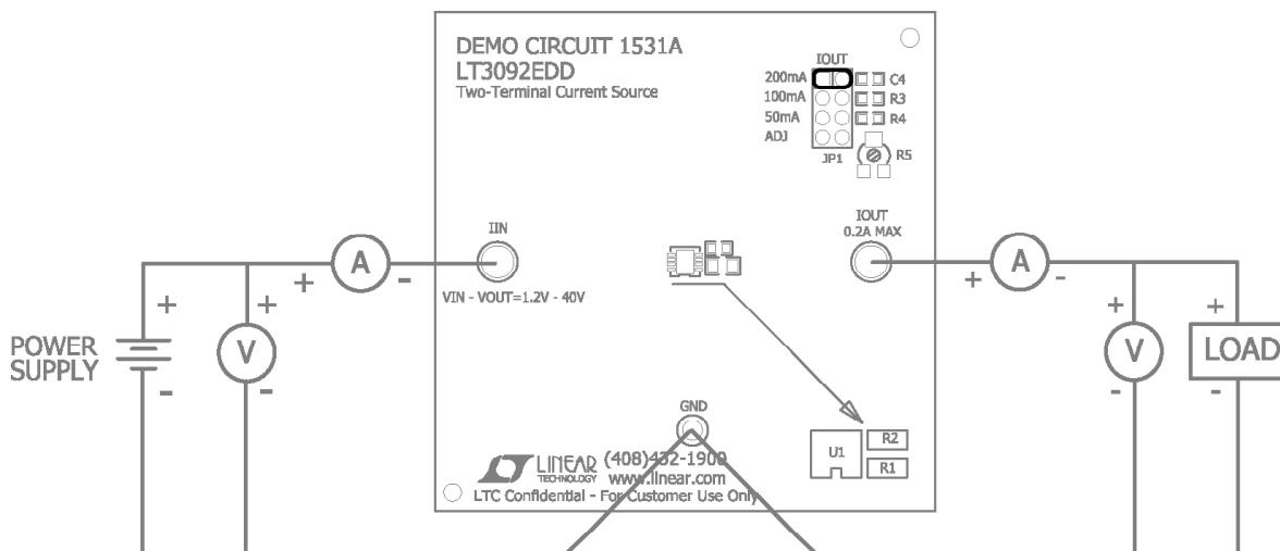
Figure 1. Proper Measurement Equipment Setup
