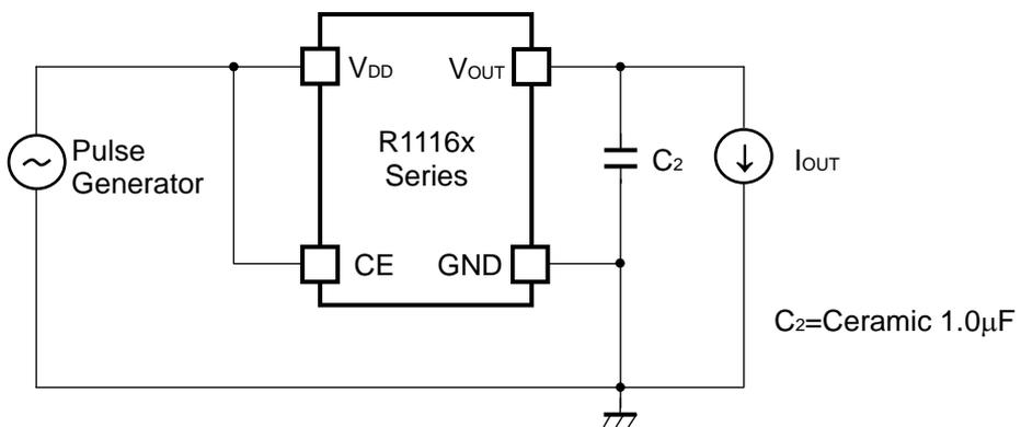
Fig.3 Ripple Rejection, Line Transient Response Test Circuit
