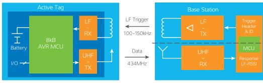
\*1) Graph shows one combined base station. Option is to split that as RX distance is much higher. So multiple trigger stations and one or few RX stations.
