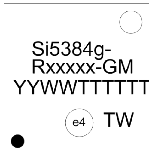
Figure 12.2. Si5384 Top Marking
