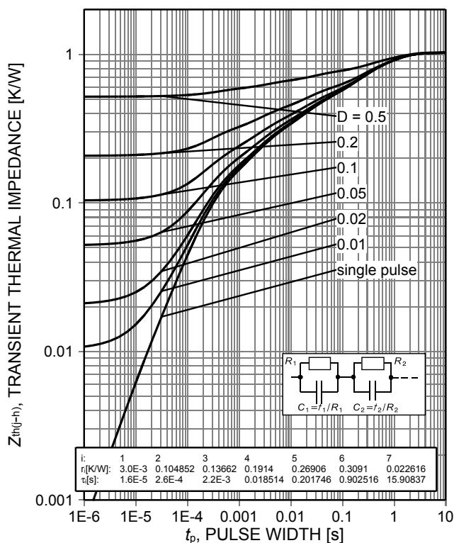
Figure 20. IGBT transient thermal impedance as a function of pulse width
