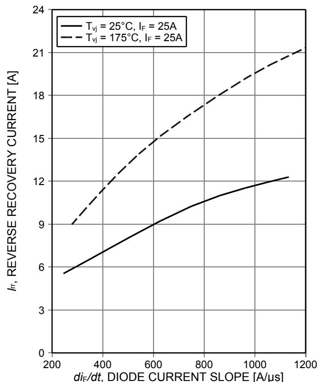
Figure 24. Typical reverse recovery current as a function of diode current slope ( $V_R=400\text{V}$ )
