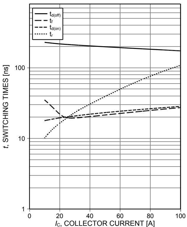
Figure 8. Typical switching times as a function of
