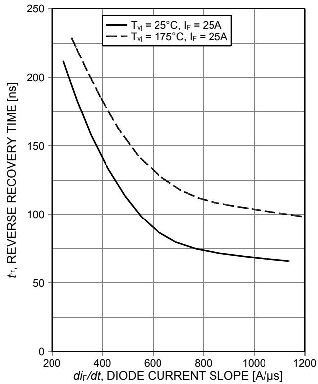
Figure 22. Typical reverse recovery time as a function of diode current slope ( $V_R=400\text{V}$ )
