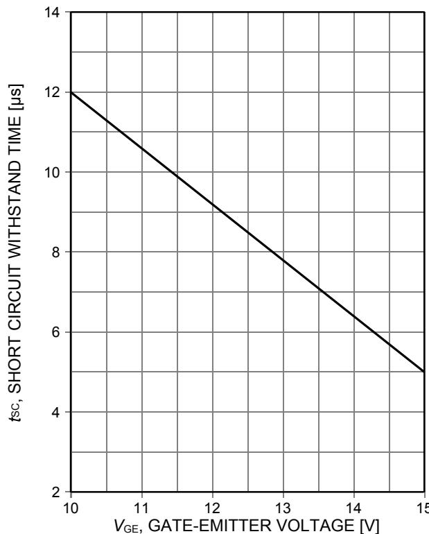
Figure 19. Short circuit withstand time as a function of gate-emitter voltage
