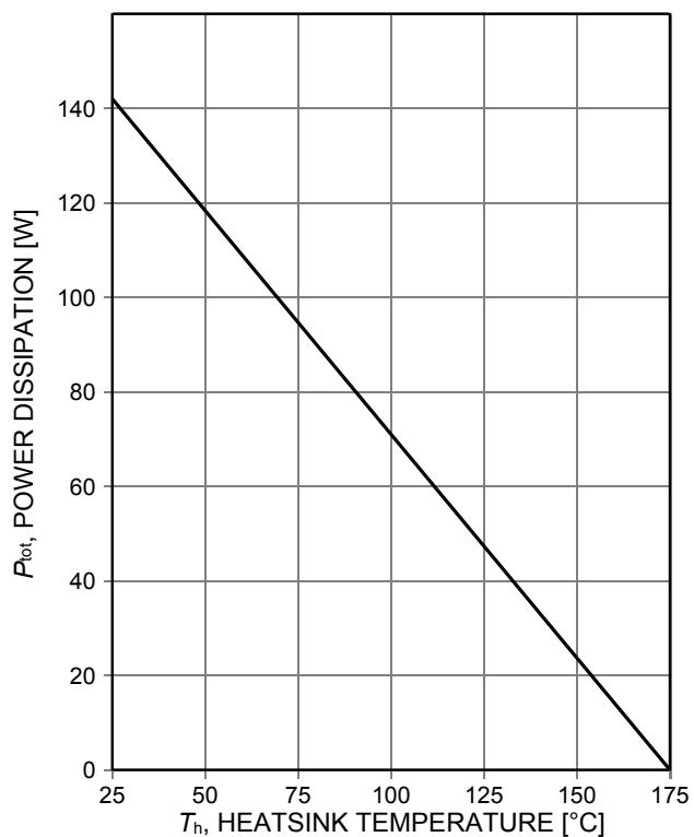
Figure 2. **Power dissipation as a function of heatsink temperature**
