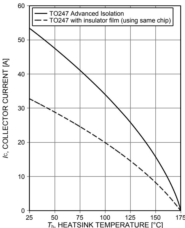
Figure 3. **Collector current as a function of heatsink temperature**
