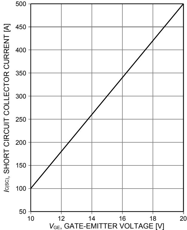
Figure 18. Typical short circuit collector current as a function of gate-emitter voltage
