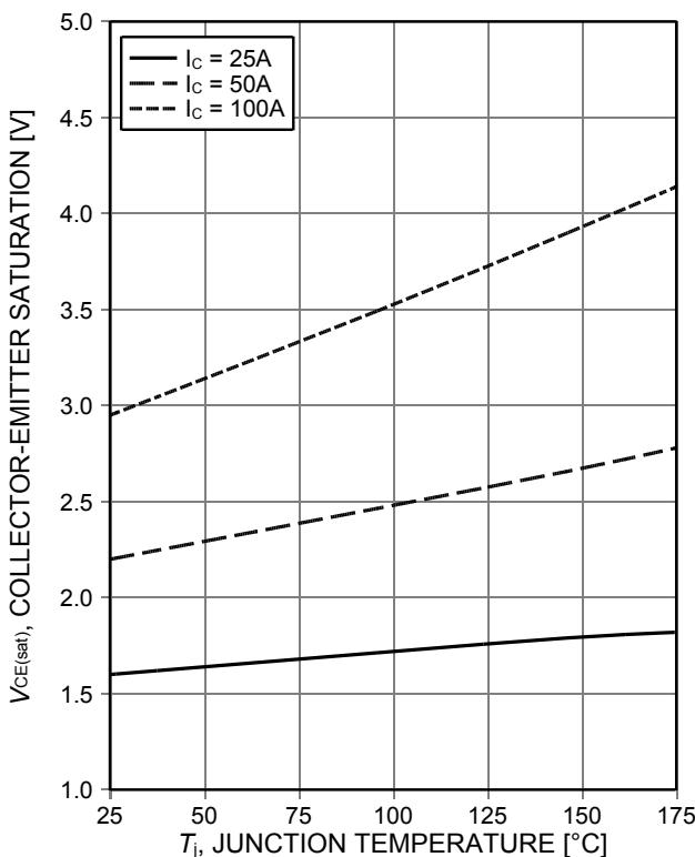
Figure 7. Typical collector-emitter saturation voltage as
