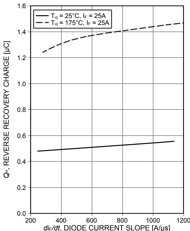
Figure 23. Typical reverse recovery charge as a function of diode current slope ( $V_R=400\text{V}$ )
