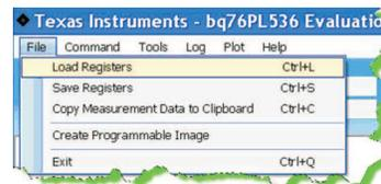
Another useful command available in this menu allows copying the current measurement data (VCn, VBRICK, and TS1, TS2, in that order) to the clipboard, and subsequent copying to a document or spreadsheet.measurements.
