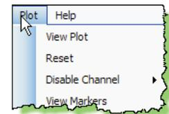
**RESET** completely resets the plotter interface, restoring display defaults and clearing all stored data.
