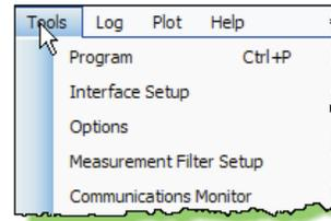
**INTERFACE SETUP** opens a dialog box that allows changing the SPI communications speed.
