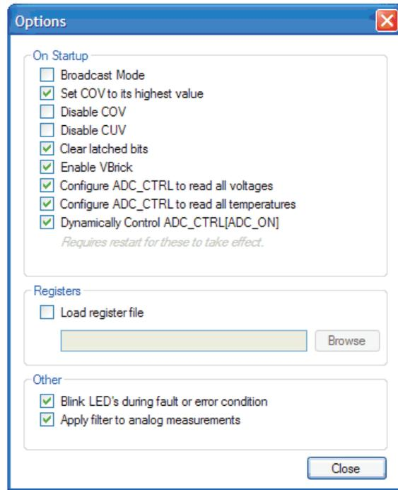
**BROADCAST MODE** when checked, brings up the interface set to broadcast messages to all devices, no data is shown. In broadcast mode, the WinGUI does not know which device to read, so no register data is displayed.
