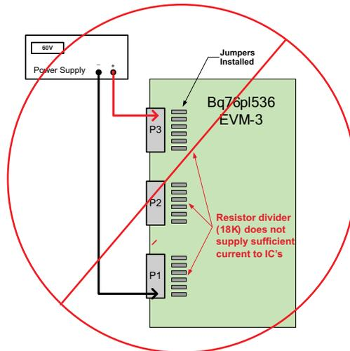
Figure 4. Incorrect Connections, Insufficient  $V_{BAT}$  Per IC
