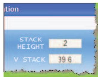
The screen automatically refreshes each time something changes. Addressing the device will cause all displayed values and registers to update. The user should see all cell voltages displayed, along with registers showing FAULT and ALERT status, DEVICE STATUS, etc.
