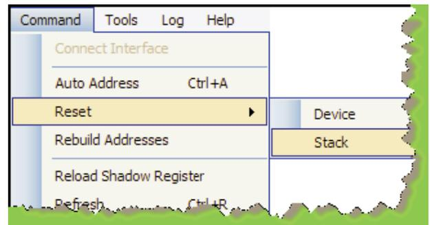
Because the part is shipped unprogrammed, the result of reloading the shadow registers is to transfer all zeros to the shadow cells, and will usually result in many ALERTS and FAULTS being triggered which are normally hidden by the GUI per the OPTION menu settings (see below).
