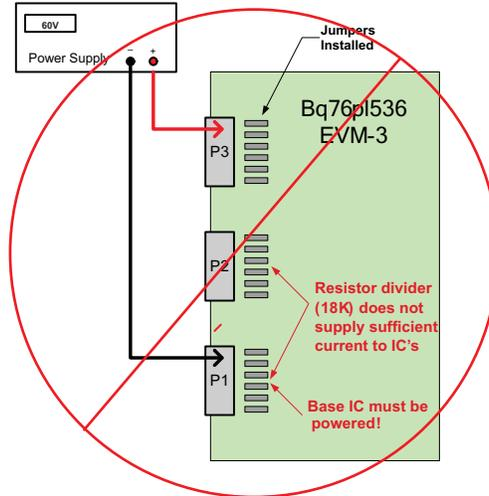
Figure 3. Incorrect Connections, Base IC Not Powered
