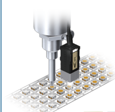
LED potting shape measurement
