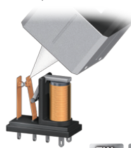
Operation inspection of relay contacts
