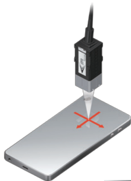
Level difference measurement of logos
