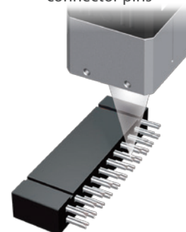
Coplanarity measurement of connector pins
