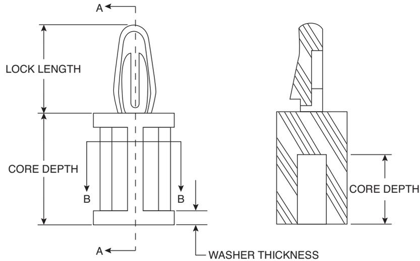
NOTE: Self Threading Posts are designed for use with a #6 self-tapping screw.
