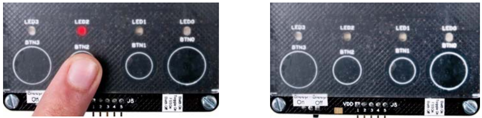
1. Touch a button; LED turns on
