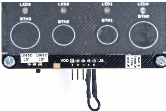
Figure 3-20. BTN1 Sensor Shorted to Ground
