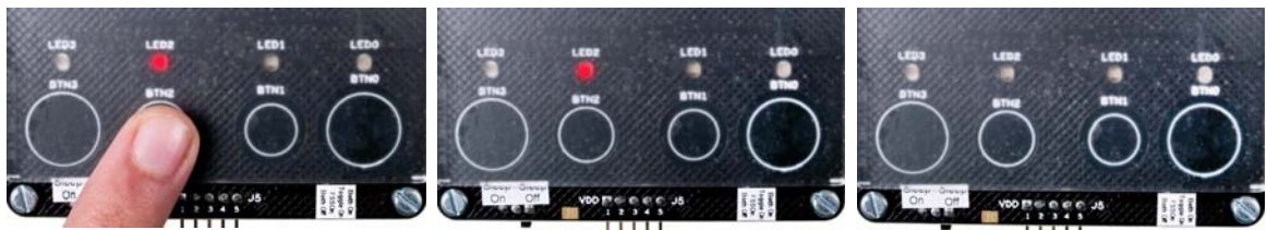
Figure 3-13. Test Sequence for Delay Off Feature
