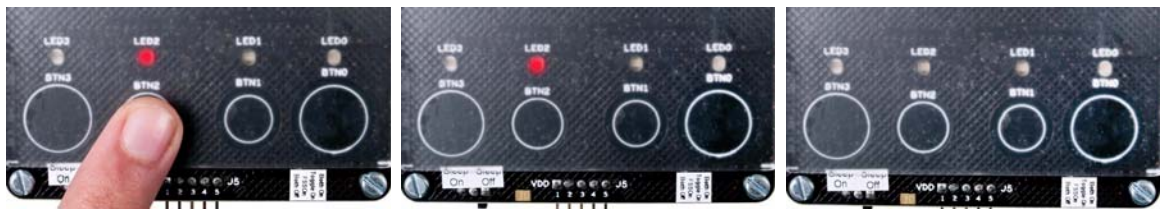
Figure 3-13. Test Sequence for Delay Off Feature
