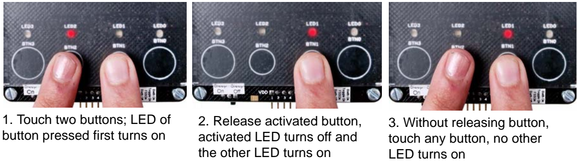
Figure 3-7. FSS Feature Test Sequence
