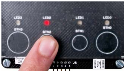
1. Touch a button; LED turns on
