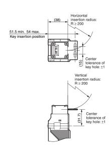
D4GL + D4DS-K1 (with Top-inserted Operation Key)
