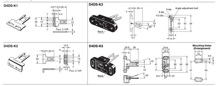
**Note:** Unless otherwise specified, a tolerance of  $\pm 0.4$  mm applies to all dimensions.
