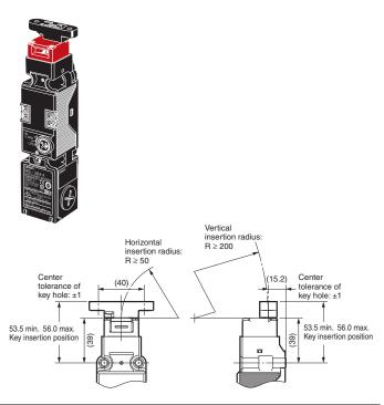
D4GL + D4DS-K5 (with Front-inserted Operation Key)
