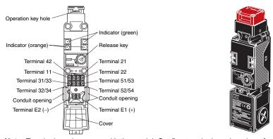
Note: Terminal numbers vary with the model. Confirm terminal numbers by referring to the cover on the back of the Switch.
