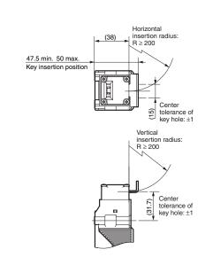
D4GL + D4DS-K2 (with Top-inserted Operation Key)
