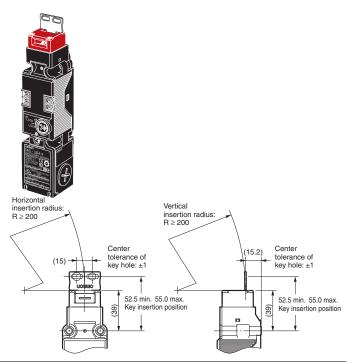
D4GL + D4DS-K2 (with Front-inserted Operation Key)
