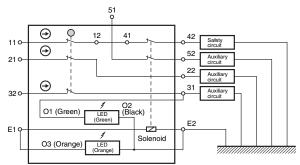
Direct opening contacts used as safety-circuit input are indicated with the → mark.
