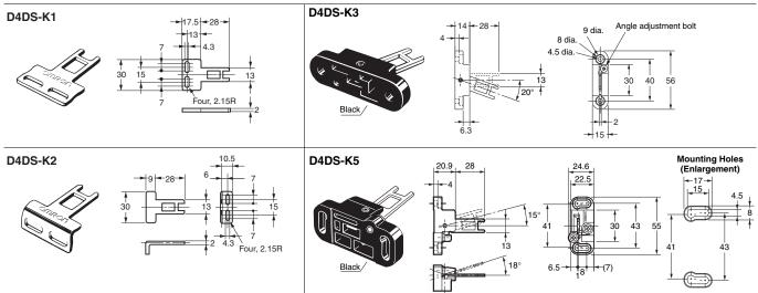
Note: Unless otherwise specified, a tolerance of  $\pm 0.4$  mm applies to all dimensions.
