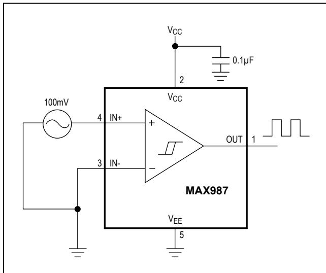
Figure 3. Zero-Crossing Detector
