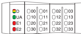
Figure 6 Local status and diagnostic indicators
