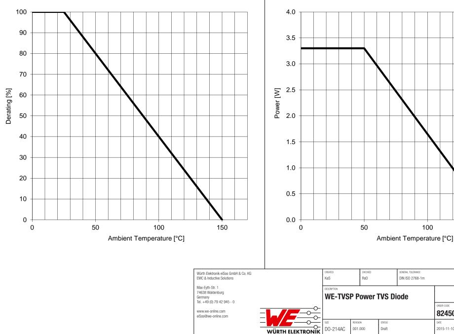
**Steady State Power Dissipation Derating**
