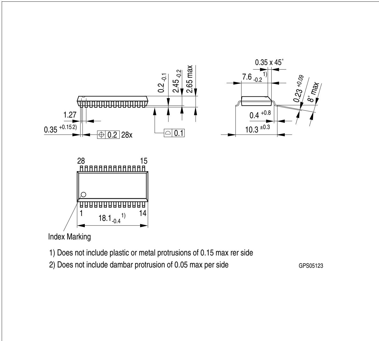
**Figure 5 PG-DSO-28-22 (Plastic Transistor Single Outline Package)**
