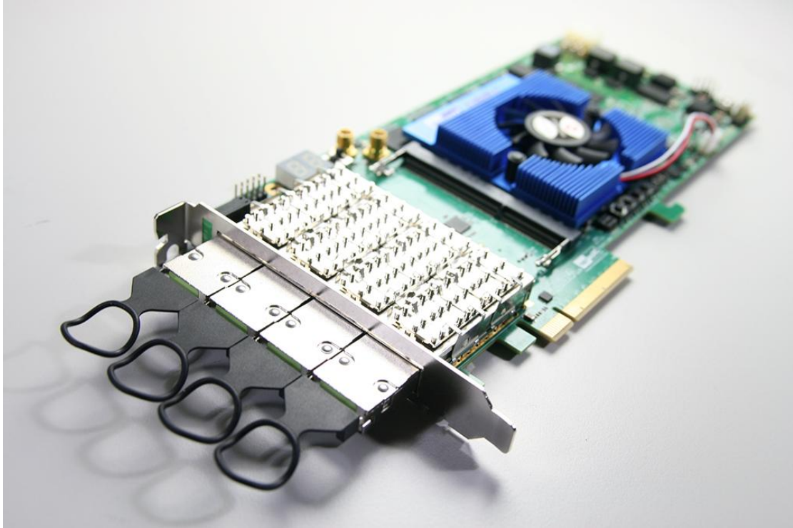
Figure 8-4 Four QSFP+ Loopback Fixtures Installed
