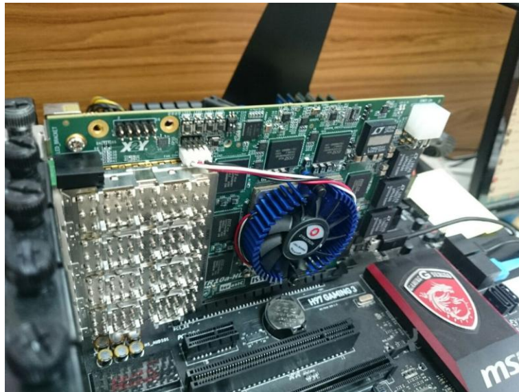
Figure 7-9 FPGA board installation on PC
