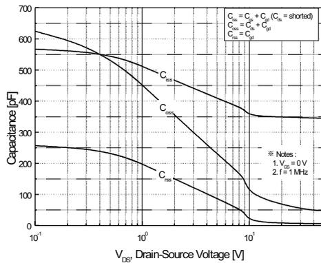
Figure 5. Capacitance Characteristics
