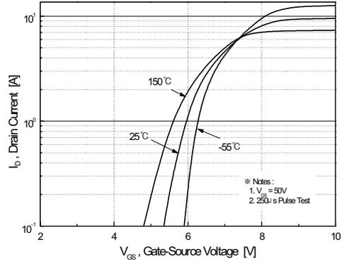
Figure 2. Transfer Characteristics
