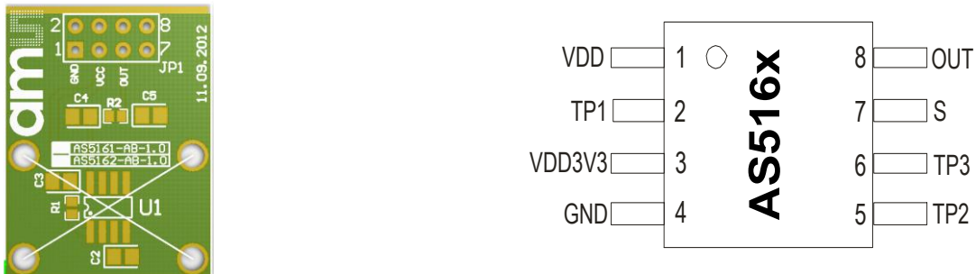
Figure 3 AS5161/AS5162 adapterboard connectors and sensor pinout
