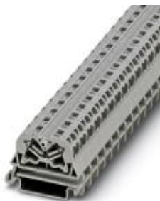
Mini feed-through terminal block, Connection method: Spring-cage connection, Cross section: 0.08 mm 2 - 4 mm 2 , AWG: 28 - 12, Width: 10.4 mm, Height: 22 mm, Color: blue, Mounting type: NS 35/7,5, NS 35/15
