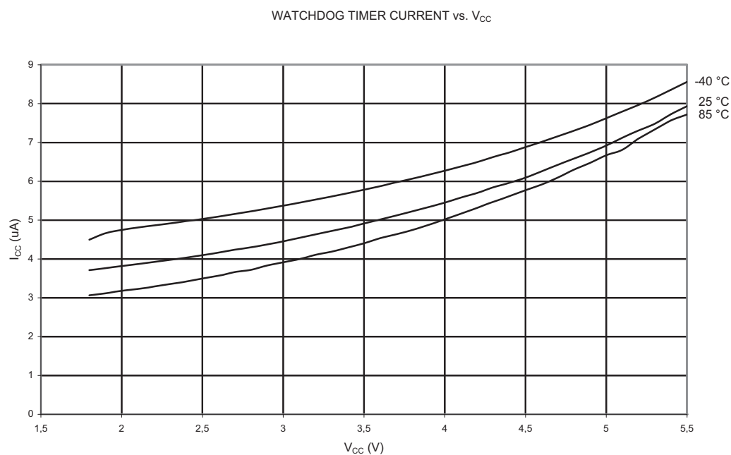
Figure 17-50. Watchdog Timer Current vs. V_{CC}
