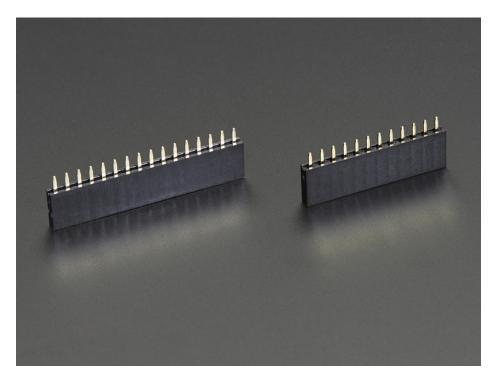
The most common method of attachment for the Proto is putting stacking or female headers on the Featherwing and then putting the Proto on top:
