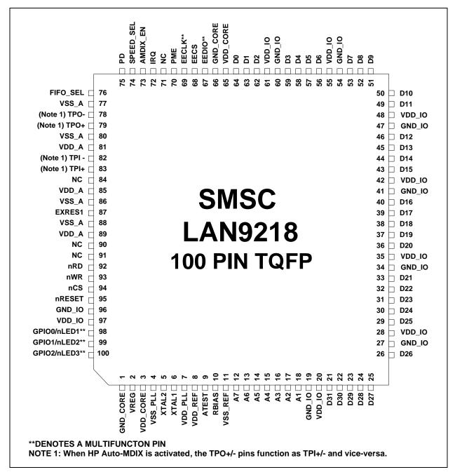
Figure 2.1 Pin Configuration (Top View)
