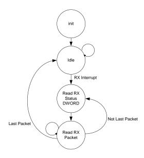
Figure 3.15 Host Receive Routine Using Interrupts
