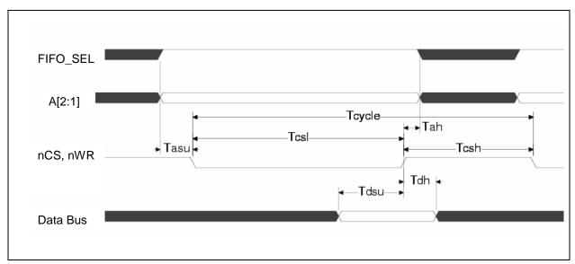
Figure 6.6 TX Data FIFO Direct PIO Write Timing
