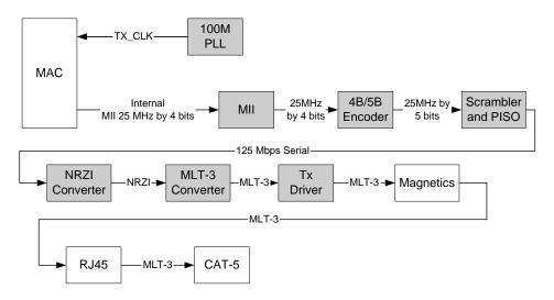
Figure 4.1 100Base-TX Data Path
