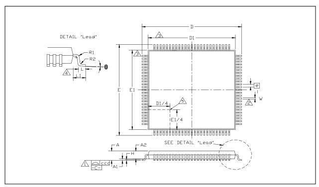
Figure 8.1 100 Pin TQFP Package Definition
