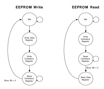
Figure 3.2 EEPROM Access Flow Diagram
