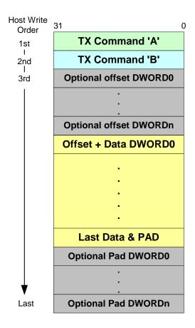
Figure 3.12 TX Buffer Format
