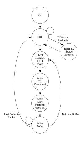
Figure 3.11 Simplified Host TX Flow Diagram
