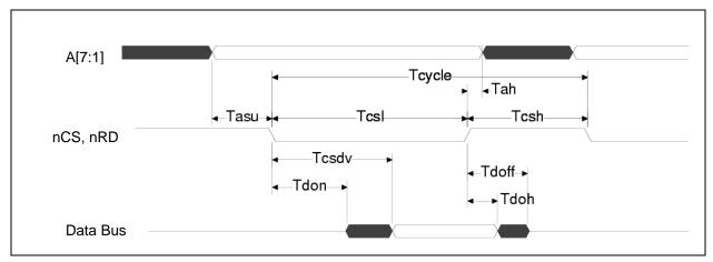
Figure 6.1 PIO Read Cycle Timing
