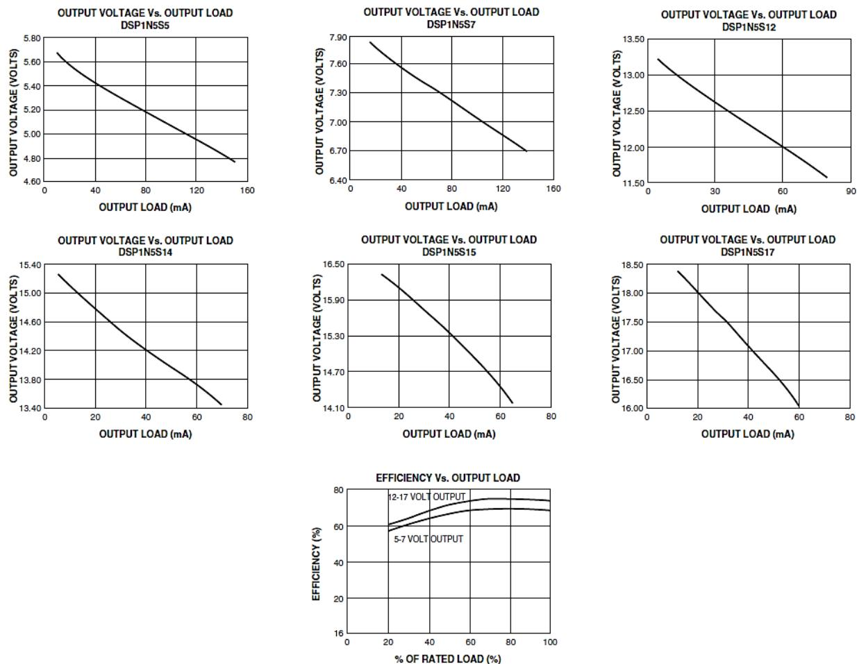
Figure 1. Typical Performance ( $T_c = 25^\circ C$ )
