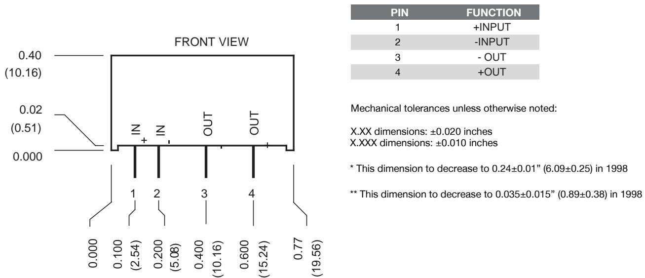
*Figure 3. Mechanical Dimensions*
