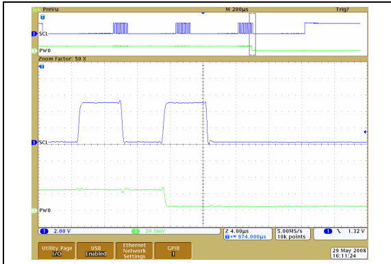
FIGURE 2-62: 50 kΩ – Low-Voltage Decrement Wiper Settling Time ( V_{DD} = 2.7\text{V} ) (1 µs/Div).
