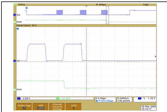
FIGURE 2-63: 50\text{ k}\Omega – Low-Voltage Decrement Wiper Settling Time ( V_{DD} = 5.5\text{V} ) ( 1\ \mu\text{s}/\text{Div} ).
