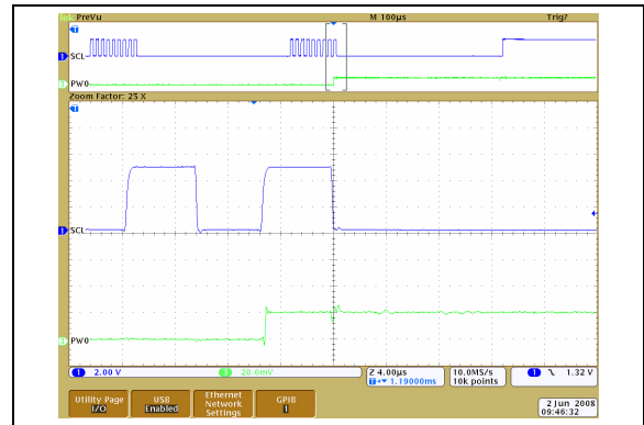
FIGURE 2-84: 100\text{ k}\Omega – Low-Voltage Increment Wiper Settling Time ( V_{DD} = 2.7\text{V} ) ( 1\ \mu\text{s}/\text{Div} ).
