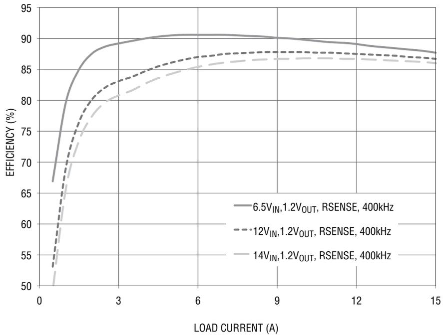
Figure 3. Typical Efficiency Curves vs Load Current with A-A (R<sub>SENSE</sub>) Board for: (A) 1.5V Rail and (B) 1.2V Rail
