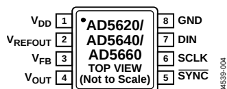
Figure 4. MSOP Pin Configuration
