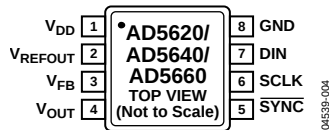
Figure 4. MSOP Pin Configuration
