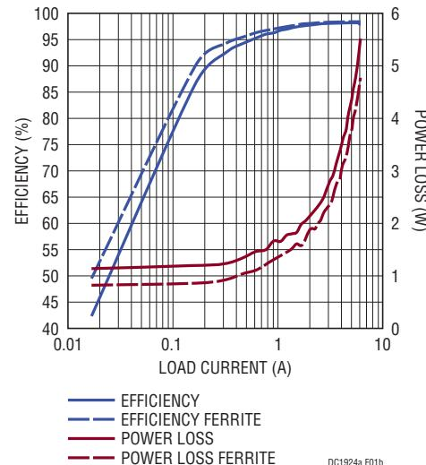
Figure 1b. Efficiency and Power Loss in CCM Buck Mode.  $V_{IN} = 56\text{V}$ . Dotted Lines Show Increased Efficiency When the Inductor Is Replaced by a Ferrite Core Inductor (Coiltronics SER2918H-223KL)
