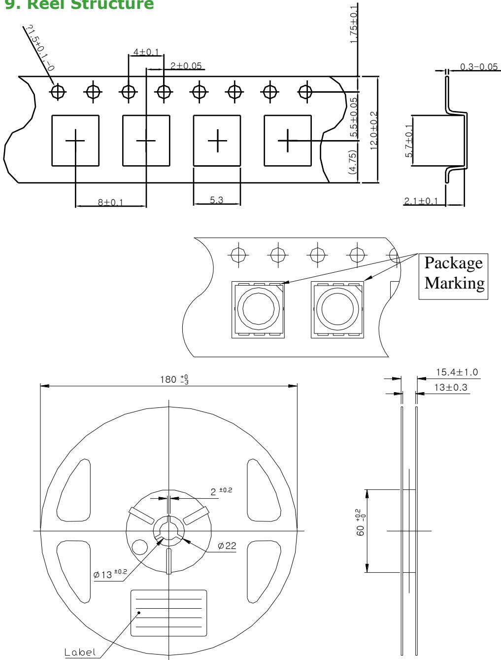
( Tolerance:  $\pm 0.2$ , Unit: mm )
