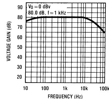
**Figure 113. Flat Amp Voltage Gain vs Frequency**
