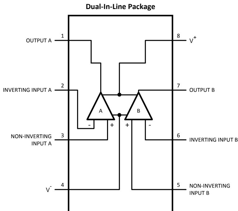
**Figure 2. 8-Lead SOIC (D Package)
