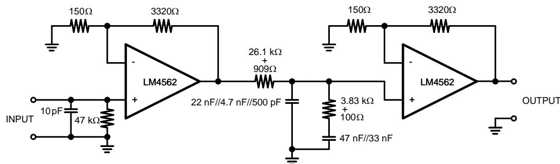
A. 1% metal film resistors, 5% polypropylene capacitors
