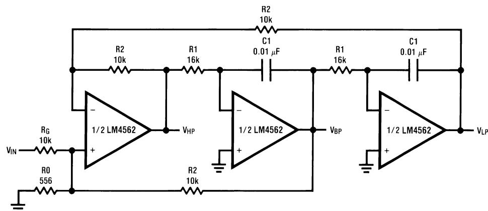
$$f_0 = \frac{1}{2\pi C_1 R_1}, Q = \frac{1}{2} \left( 1 + \frac{R_2}{R_0} + \frac{R_2}{R_G} \right), A_{BP} = Q A_{LP} = Q A_{LH} = \frac{R_2}{R_G}$$
