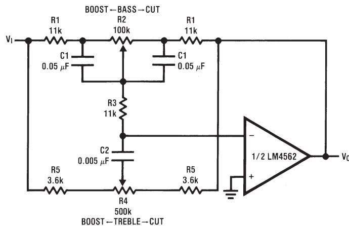
$$f_L \approx \frac{1}{2\pi R_2 C_1}, f_{LB} \approx \frac{1}{2\pi R_1 C_1}$$
