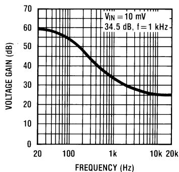
Figure 115. NAB Preamp Voltage Gain vs Frequency
