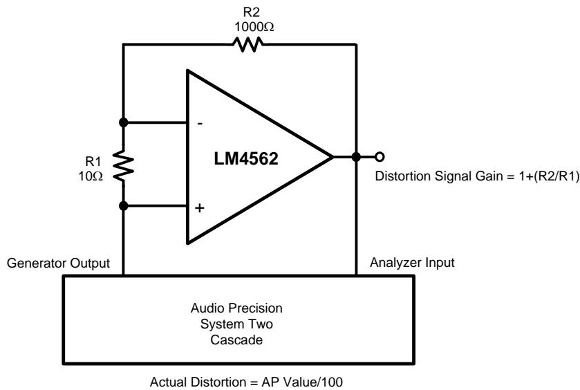
**Figure 110. THD+N and IMD Distortion Test Circuit**
