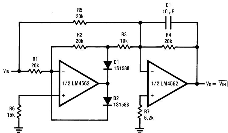
**Figure 122. AC/DC Converter**
