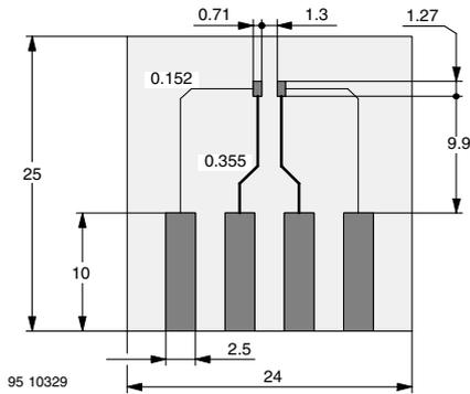
Figure 5. Board for  $R_{thJA}$  definition (in mm)
