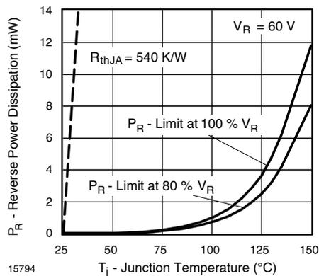
Figure 1. Max. Reverse Power Dissipation vs. Junction Temperature
