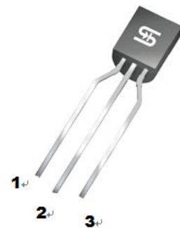
1. Collector 2. Base 3. Emitter TO-92 Plastic Package
