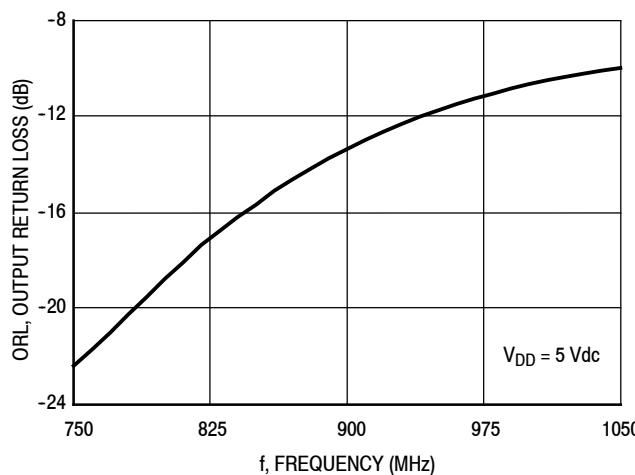
Figure 17. Output Return Loss (S22) versus Frequency
