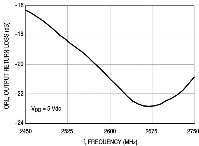
Figure 25. Output Return Loss (S22) versus Frequency
