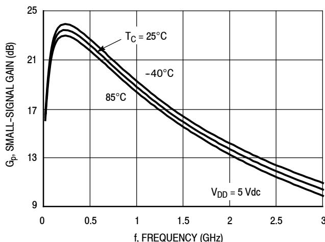
**Figure 2. Small-Signal Gain (S21) versus Frequency <sup>(1)</sup>**
