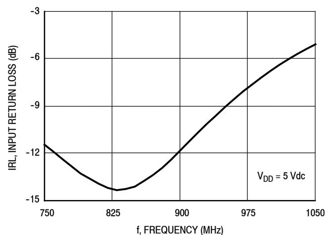
Figure 16. Input Return Loss (S11) versus Frequency
