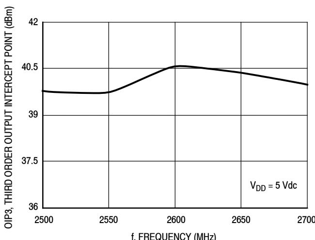
Figure 27. Third Order Output Intercept Point versus Frequency
