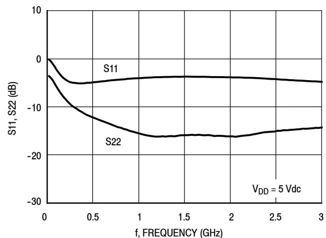
**Figure 3. Input/Output Return Loss versus Frequency <sup>(1)</sup>**
