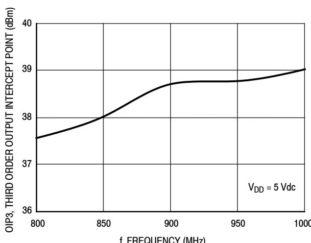
Figure 19. Third Order Output Intercept Point versus Frequency
