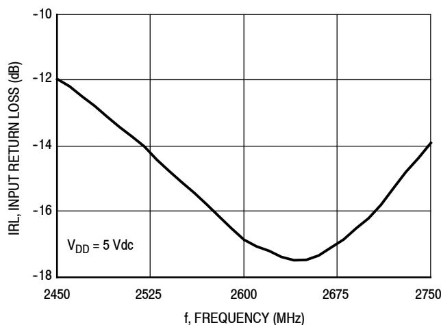
Figure 24. Input Return Loss (S11) versus Frequency
