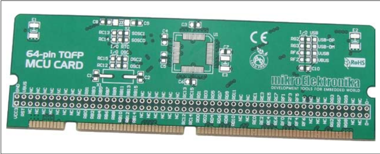
Figure 3: Empty 64-pin MCU card
