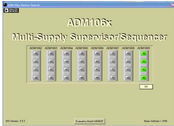
Figure 28 four ADM1069 devices at addresses 98 9A 9C and 9E
