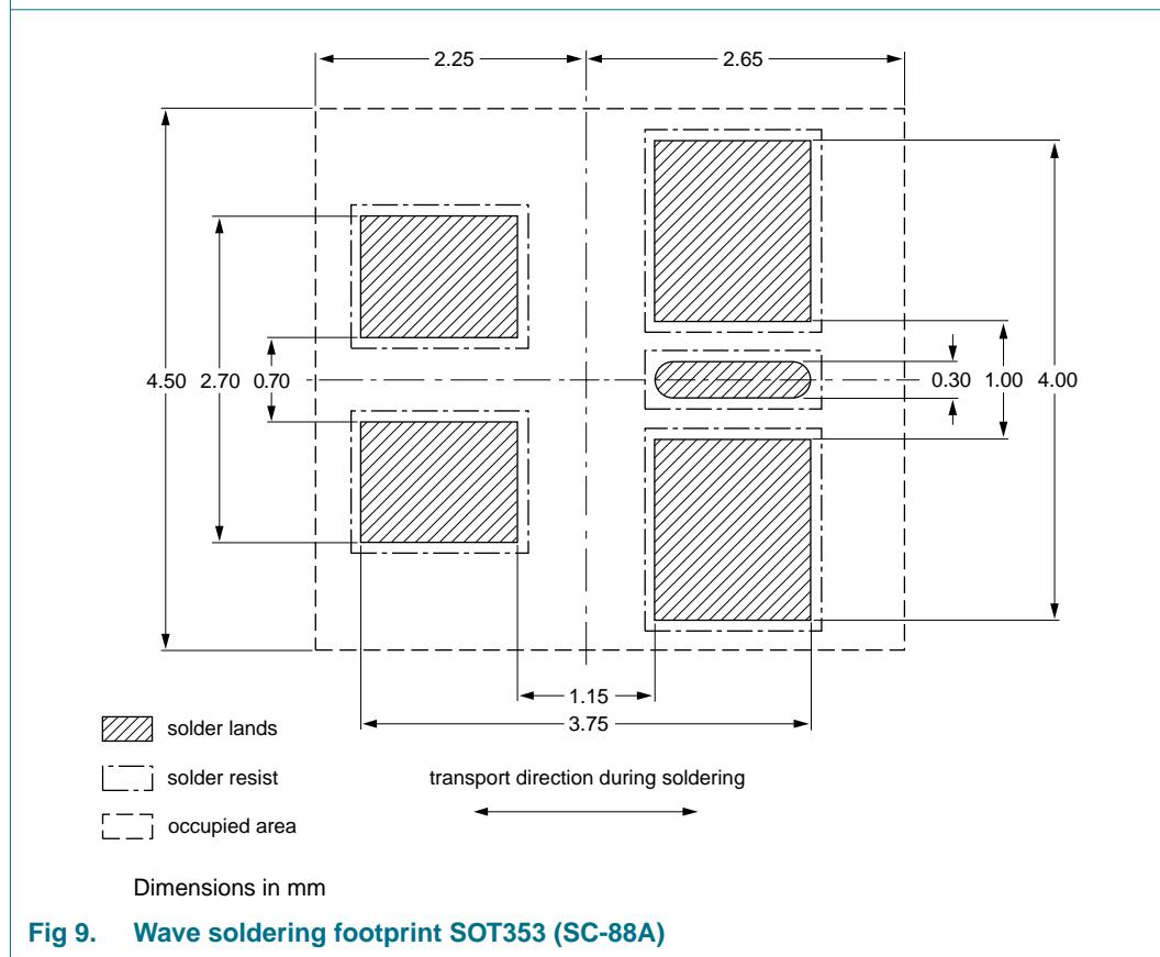
**Fig 9. Wave soldering footprint SOT353 (SC-88A)**
