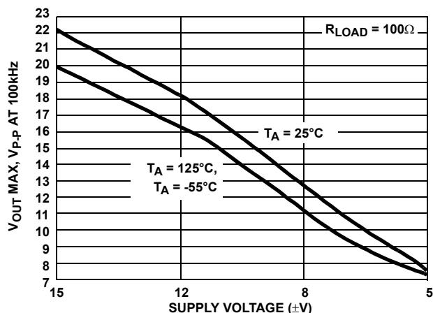
FIGURE 14. V<sub>OUT</sub> MAXIMUM vs V<sub>SUPPLY</sub>
