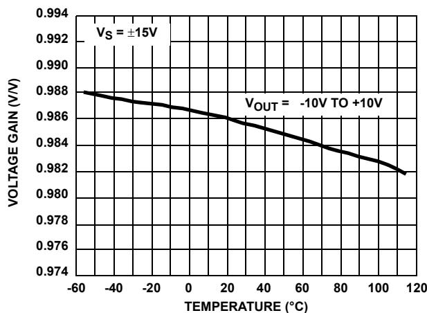
FIGURE 6. VOLTAGE GAIN vs TEMPERATURE ( $R_L = 100\Omega$ )
