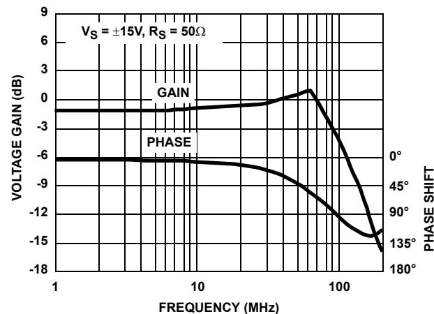
FIGURE 5. GAIN/PHASE vs FREQUENCY ( $R_L = 50\Omega$ )
