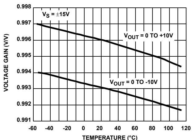
FIGURE 7. VOLTAGE GAIN vs TEMPERATURE ( $R_L = 1k\Omega$ )
