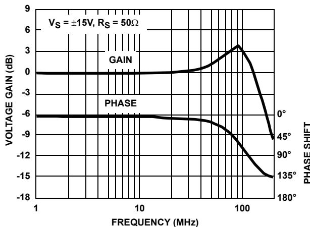
FIGURE 4. GAIN/PHASE vs FREQUENCY ( $R_L = 1\text{k}\Omega$ )
