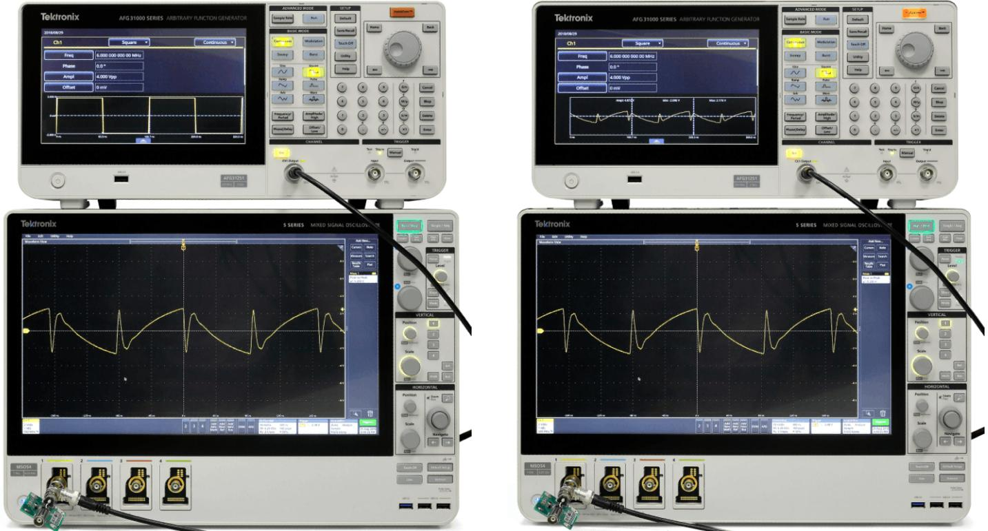
With InstaView turned off, the AFG31000 works like a traditional function generator. Due to an impedance mismatch, the AFG display shows a different waveform from the one observed at the DUT.
