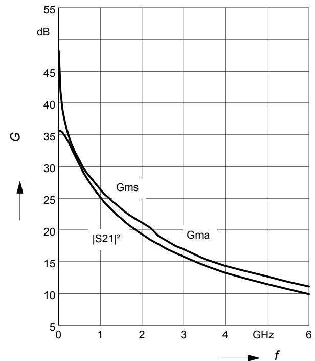
**Power gain  $G_{\text{ma}}, G_{\text{ms}} = f(I_C)$**
